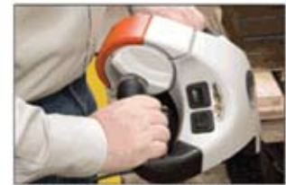
Auto reversing "belly bump" switch protects against operator accidents while working in tight quarters.
