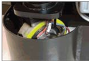
Smooth polyurethane drive wheel is fully shrouded to protect operators' feet
