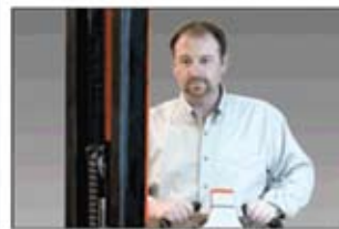
Narrow mast and offset design provide workers a clear view with no "blind spots"
